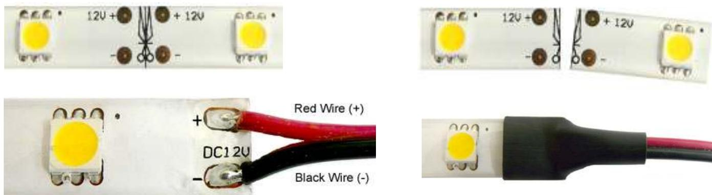
You need to cut the Strip along the line with the 4 solder pads on either side of the cut.
